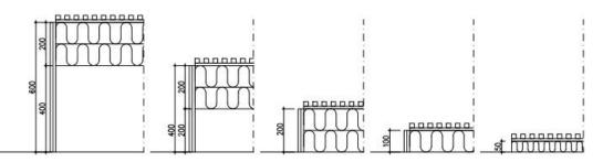
Figure 7. Absorber thicknesses measured with the slat sequences. The absorbent layer consisted of 100 mm polyester fiber wool (Ewona, 20 kg/m2) and 100 mm mineral wool (30 kg/m2), polyester being on the top. 50 mm measurement was performed with mineral wool.
