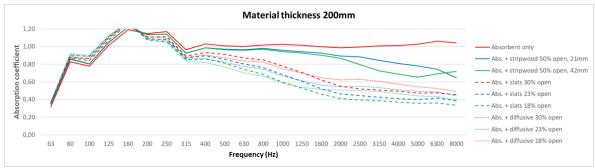
Figure 12. The absorption of absorbent only and different slat structures with 200 mm material thickness.
