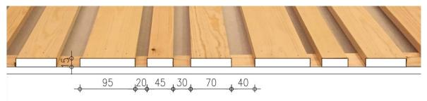
Figure 4. Slat sequence with 15mm thick slats and 30 % open area.
