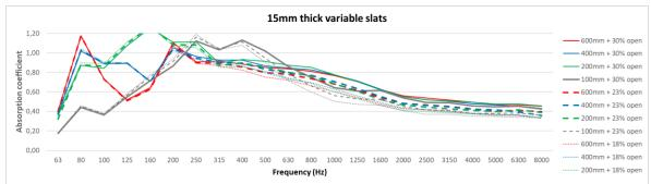
Figure 16. The absorption of 15 mm variable slats with 30 %, 23 % and 18 % open area.
