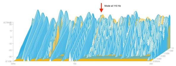
Figure 9. The FFT waterfall of the reverberation room between 20-200 Hz from one microphone position. The empty room is shown in blue and the room with 600 mm absorbent on the floor is shown in yellow.
