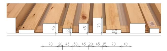
Figure 5. Slat sequence with diffusive slats and 30 % open area.
