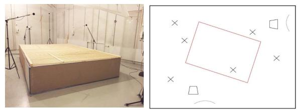
Figure 2. On the left, an image from the reverberation room showing the measurement setup. On the right, the measurement setup. Microphone positions are marked with x and loudspeaker positions with trapezoid, whose wider side shows the facing direction of the loudspeaker. Curved lines present the convex surfaces used to diffuse the sound from loudspeakers. The sample area is shown with red line.
