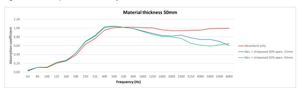
Figure 14. The absorption of absorbent only and different slat structures with 50 mm material thickness.
