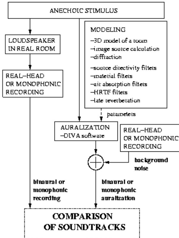
Fig. 4. A framework for perceptual evaluation of auralization systems.
