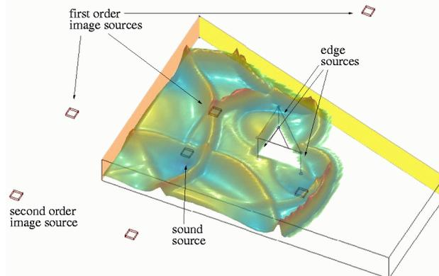
Fig. 1. An example of the sound field decomposition into elementary waves modeled with the image-source method. The illustration is done by computing an impulse response in each pixel and by plotting the time moment of 680<sup>th</sup> sample that corresponds to 14.2 ms in time.
