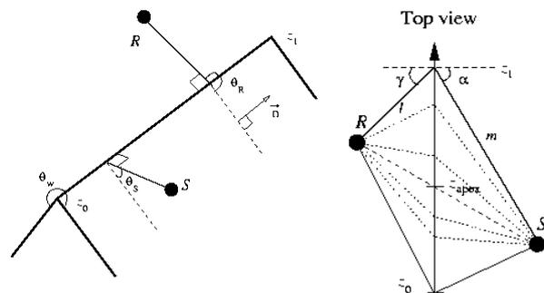
Fig. 3. Geometry of a finite wedge. The positions of source  $S$  and receiver  $R$  are indicated in cylindrical coordinates. On the right, sound paths via edge points  $z_0$  and  $z_1$  are indicated by solid lines, the least-time sound path via the apex point  $z_{\text{apex}}$  is depicted with dashed line and some other sound paths are illustrated with dotted lines.
