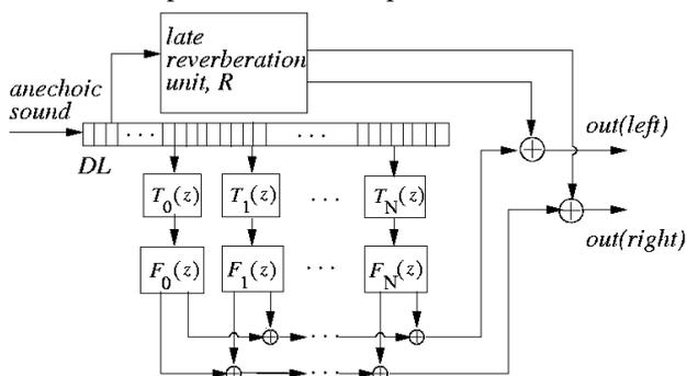
Fig. 2. Signal processing structure for auralization based on sound field decomposition.
