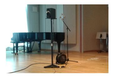
Figure 2: SRIR measurement set-up on stage
